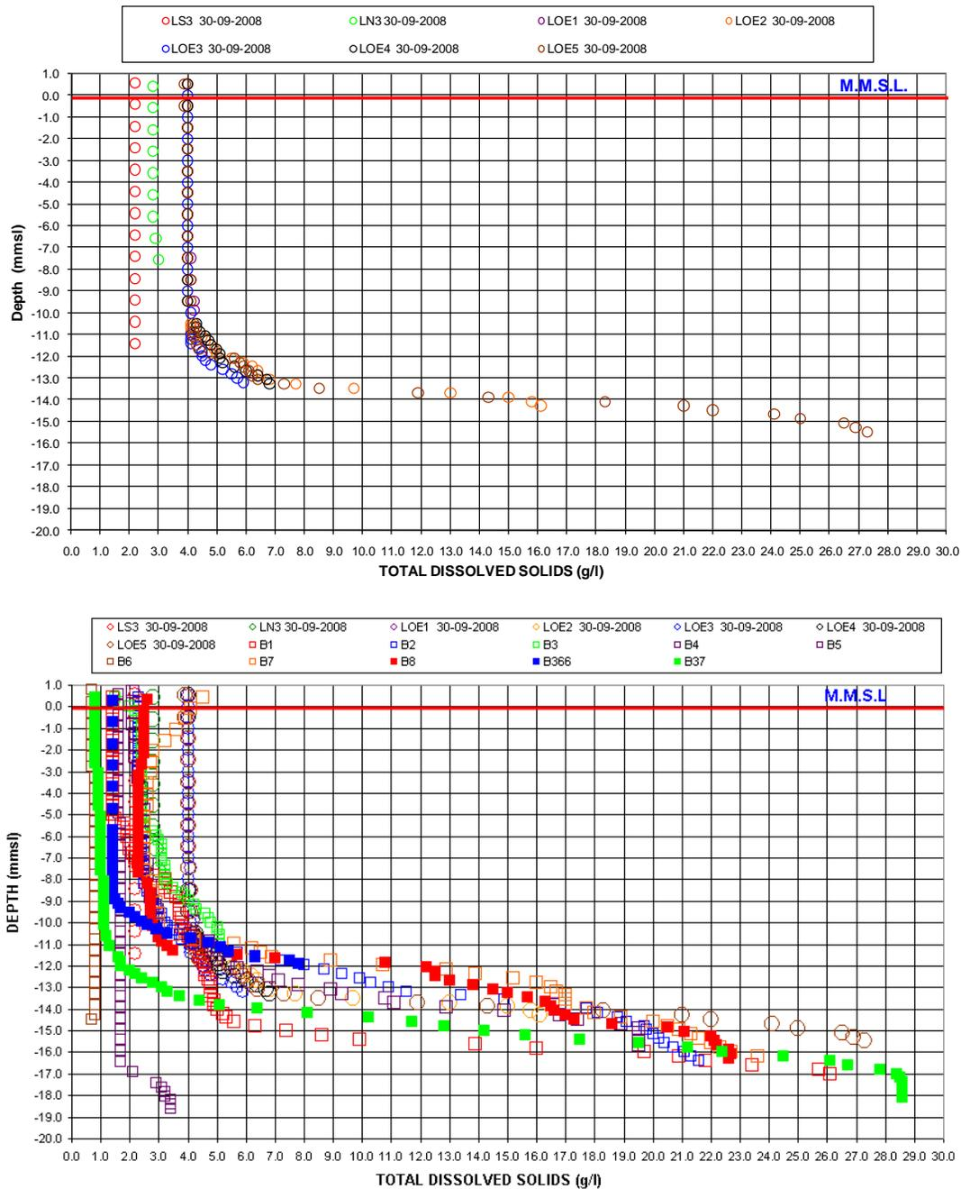
Figure 6. Total dissolved solids in the lagoons and boreholes of Mitza.
