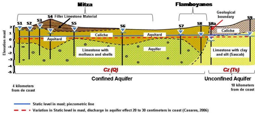
Figure 4: Hydrogeological section N-S.
