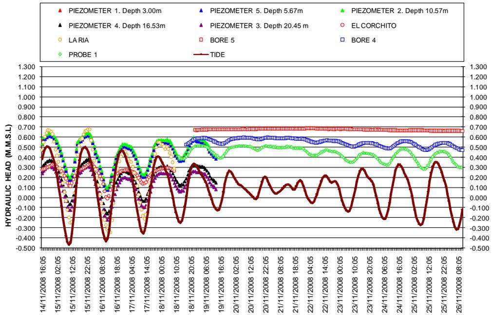
Figure 9: Variation of the hydraulic potential and tidal monitoring points (14 Nov to 01 Dec-08).
