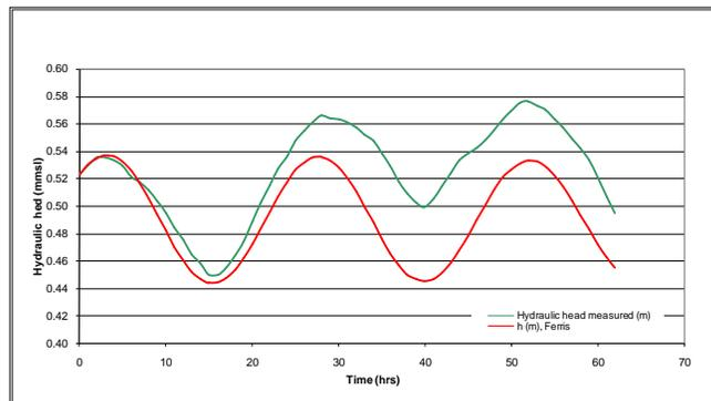
Figure 10: Graph match for the calculation of hydraulic conductivity
