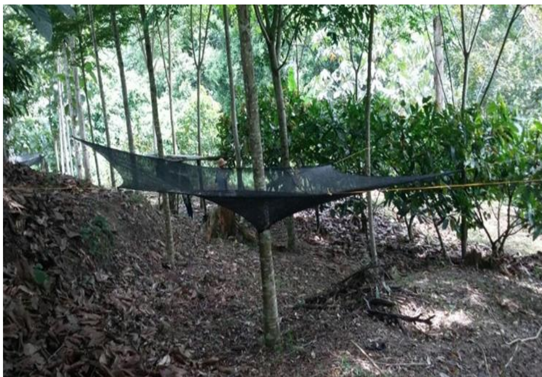
Figure 2. Modified leaf litter trap with mesh collection surface installed in the cacao understory for monthly quantification of litterfall biomass and nutrient cycling. [Photograph by Eliana Báez].
